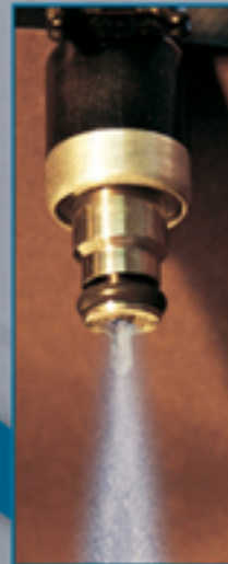
Cleaned fuel injector
