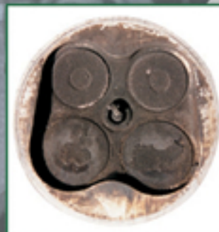
Dirty, inefficient combustion chamber
